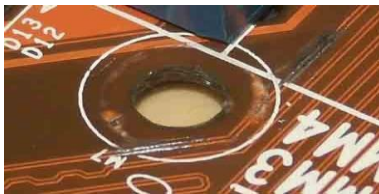
Assembly screw shorting electrical connection on PCB
