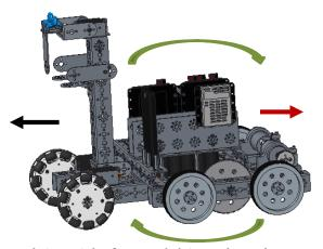
Both joysticks forward drives the robot forward
