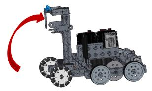
B button moves the mechanism up
