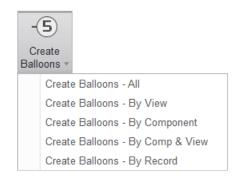
Numbered balloons connected to each of the parts listed in the bill of materials appear in the drawing.
