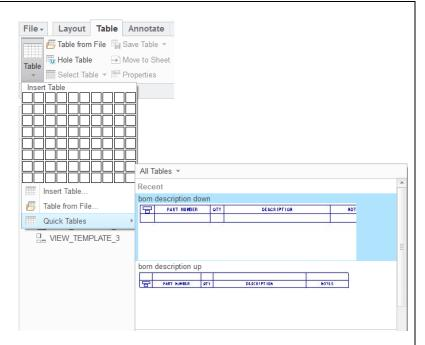
In the example, the table is placed in the top-right corner. It extends beyond the drawing. We will remove the Description and Notes columns in the next step.
