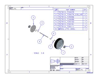
The assembly drawing provides a visual record of all of the parts in your wheel assembly. You can make several different assembly drawings to document each subassembly as well as your entire system design.
