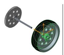
Selected parts and groups of parts can move along the three axes.
