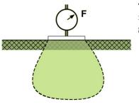
The sub-base constant k (modulus of reaction) is typically obtained from plate load tests. This 'k' value must be achieved below the grade slab before the casting of the slab.
