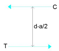
Calculation of the nominal moment is easily computed by multiplying either the compressive force, C, or tension force, T, by the moment arm. Either method is effective.
