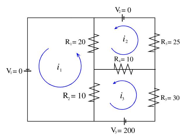
A simple electrical network contains a number of resistances and three source of electromotive force (3 batteries) as shown above.
