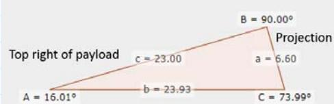
The shadow projects from each side of the payload 6.602 in along the bottom surface. This gives the shadow a radius of 1.727 inches, or a circular projection of 3.545 inches on the bottom surface. We can now compute the view factor.
