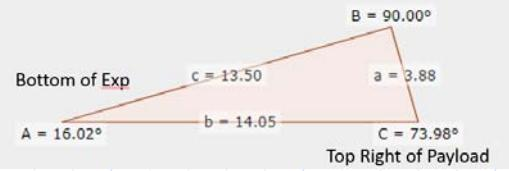
$$AT := \left( \arccos \left( \frac{(bT)^2 + (cT)^2 - (aT)^2}{2 \cdot bT \cdot cT} \right) \right) \quad AT = 16.0154 \text{ deg}$$
