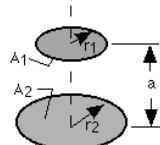
$$r_{251} := \frac{9.75 \text{ in}}{2} \quad r_{252} := \frac{2 \text{ in}}{2} \quad a_{25} := \frac{23 \text{ in}}{2} - \frac{4 \text{ in}}{2} \quad R_{251} := \frac{r_{251}}{a_{25}} \quad R_{252} := \frac{r_{252}}{a_{25}}$$
