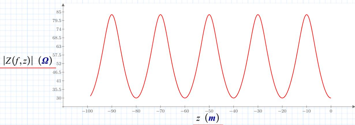
**Fig. 3.1.3 Impedance as a function of distance**
