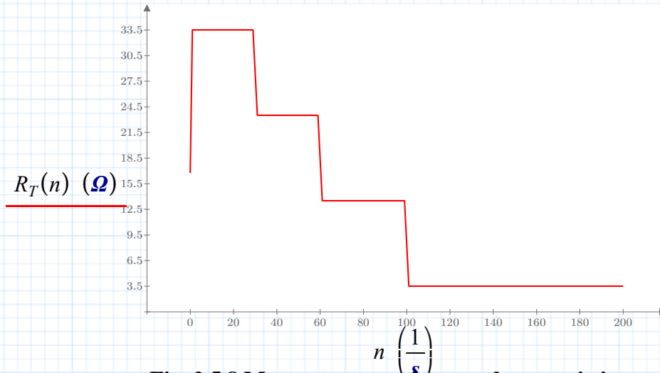
Fig. 2.5.8 Motor starter resistance characteristics
