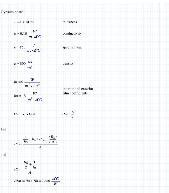
Note that the gypsum board is modeled by a thermal capacitance connected to two resistances, each equal to half the total thermal resistance Rg. Only the thermal capacity of the gypsum board is considered in this problem because it is the interior layer, and it thus stores or releases heat due to thermal changes in the room much more than the outer layers. For a more accurate analysis of transient heat transfer, the finite difference method may be employed (Section 3.3).
