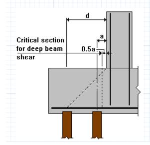
Shear spans in the X and Y directions are one-half the distances between the closest pile row and the face of the pier (See ACI 318, Chapter 11 Notation, and 11.8):
