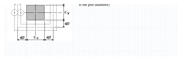
Perimeter of critical section for slabs and footings expressed as a function of d (ACI 318, 11.12.1.2):
