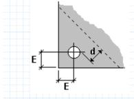
Critical Section for Beam Shear for 1 corner pile
