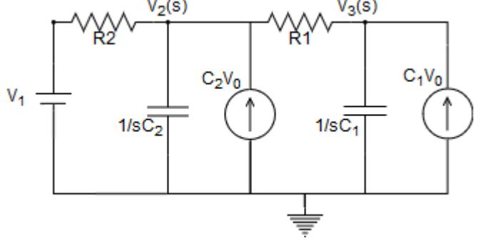
$$\frac{V_1 - V_2(s)}{(R_2 + R_g)} = sC_2 V_2(s) + C_2 V_o + \frac{V_2(s) - V_3(s)}{R_1} \text{ solve, } V_2(s) \rightarrow \frac{\frac{V_3(s)}{R_1} - C_2 V_o + \frac{V_1}{s(R_2 + R_g)}}{\frac{1}{R_2 + R_g} + \frac{1}{R_1} + C_2 s}$$
