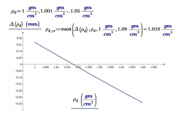
Fig. 23.7. Stability chart of the ship depending on water density
