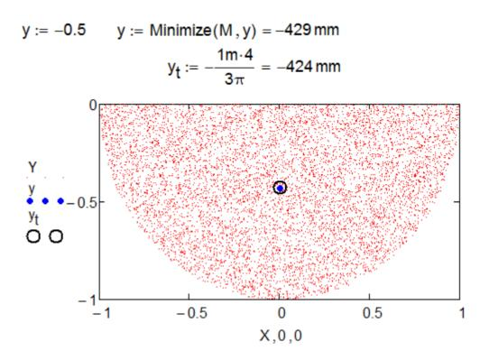
Fig. 23.9. Verification of the approximate calculation of the center of mass of a plane figure
