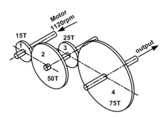
The *gear-train ratio* for the first gearset
