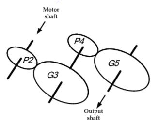
Propose 2 gear combinations for Gear 3 and 5 if the total reduction ratio is 24. You are constrained to a maximum speed ratio not exceeding 10 at each gearset. Your answers must be tabulated in the format given below.
