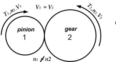
Gear-train ratio for a set of 2 gears  $e = \frac{n_2}{n_1} = \frac{N_1}{N_2}$
