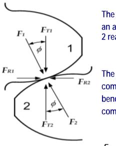
The pinion tooth 1 applied force  $F_1$  against the gear teeth 2 at an angle equal to pressure angle. For equilibrium, gear teeth 2 reacts with equal force  $F_2$  against pinion teeth 1 and so
