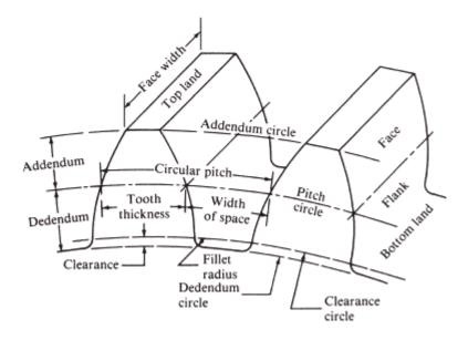
Facewidth : width of the gear toothaddendum : distance between the top land to the pitch circlededundum : distance between the pitch circle to the bottom of the gear
