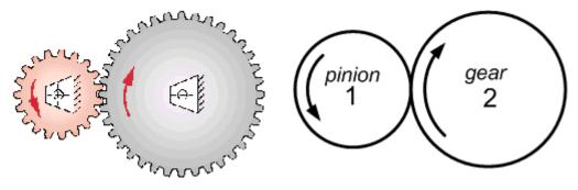
A pair of gears (pinion and gear) can be represented by 2 circles. The diameter of the two circles are based on the <u>pitch circle diameters</u> of the mating gears.
