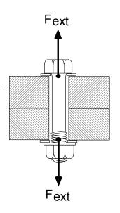
$$\begin{split} \Delta F_{j} &\coloneqq F_{ext} \begin{pmatrix} K_{j} \\ \overline{K_{j} + K_{bolt}} \end{pmatrix} \qquad \Delta F_{j} = 5.232 \times 10^{3} \, \text{lbf} \\ \Delta L_{j} &\coloneqq \frac{\Delta F_{j}}{K_{j}} \qquad \Delta L_{j} \\ \Delta F_{bolt} &\coloneqq \Delta L_{j} \\ \Delta F_{bolt} &\coloneqq K_{bolt} \cdot \Delta L_{bolt} \qquad \Delta F_{bolt} = 2.768 \times 10^{3} \, \text{lbf} \end{split}$$
