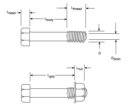
Lgrip -- Grip length Lnut -- Length of the nut Esmin -- Minimum pitch diameter of the threads D -- Nominal diameter of the threads Lhead -- Lenngth of the head of the bolt Lbody -- Length of the unthreaded portion of the shank Lthread -- Length of the threaded portion of the bolt
