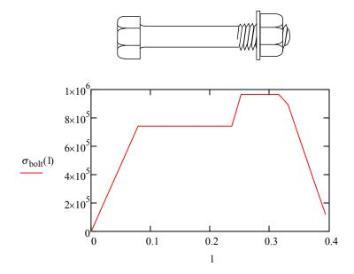
The force (F) that a bolt can support before the shank (as opposed to the threads)
