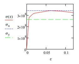
This plot shows the stress/strain behavior of the bolt material.
