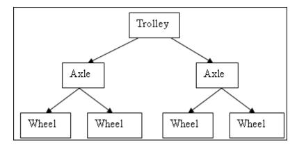
However, the 2 axles are identical to each other as are the wheels except for their locations. As each wheel may have a lot of shared information, we ensure that this information is stored in memory and build this assembly up from components. The component acts as a storage vessel in a file structure. It is used to hold properties which store or reference the actual data or other subcomponents.
