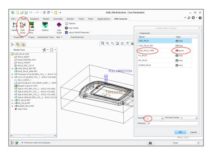
Even when create a single cavity mold, we recommend to create a copy of the original Core? Cavity insert with the Multi Cavity function.
