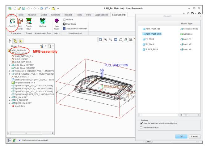
In the past many users have used the classifying of the project to put components to the fixmoving half. This is not the correct way to do it.
