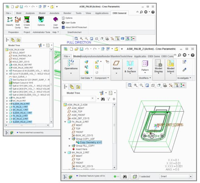
Copies of the Insert models are added to the insert-assembly
