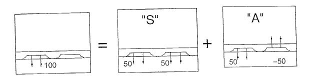
As indicated above, we can superpose the results for the original problem from 2 analyses of a symmetrically loaded structure and a anti-symmetrically loaded structure ( denoted by "S" and "A" ) .
