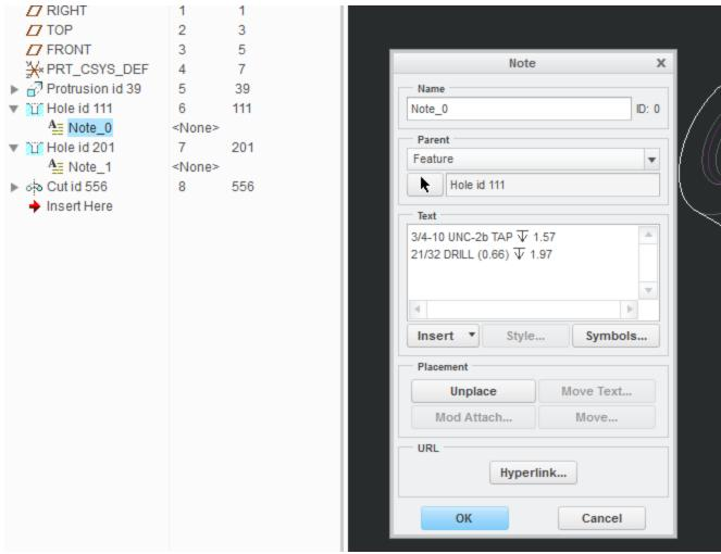
And when creating this hole from new, Creo automatically adds the fractional internal thread note:
