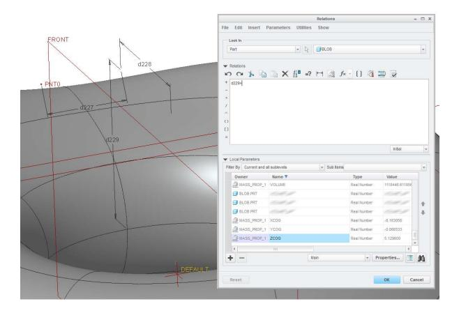
Now we need to add the analysis parameter from step #2. This will make the point offsets be controlled by the distances calculated with the mass analysis.
