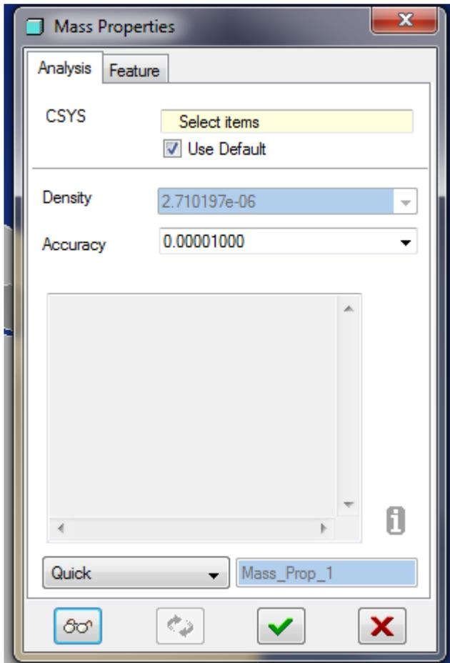
6. When the Mass Properties window opens up, press the icon with the eyeglasses.
